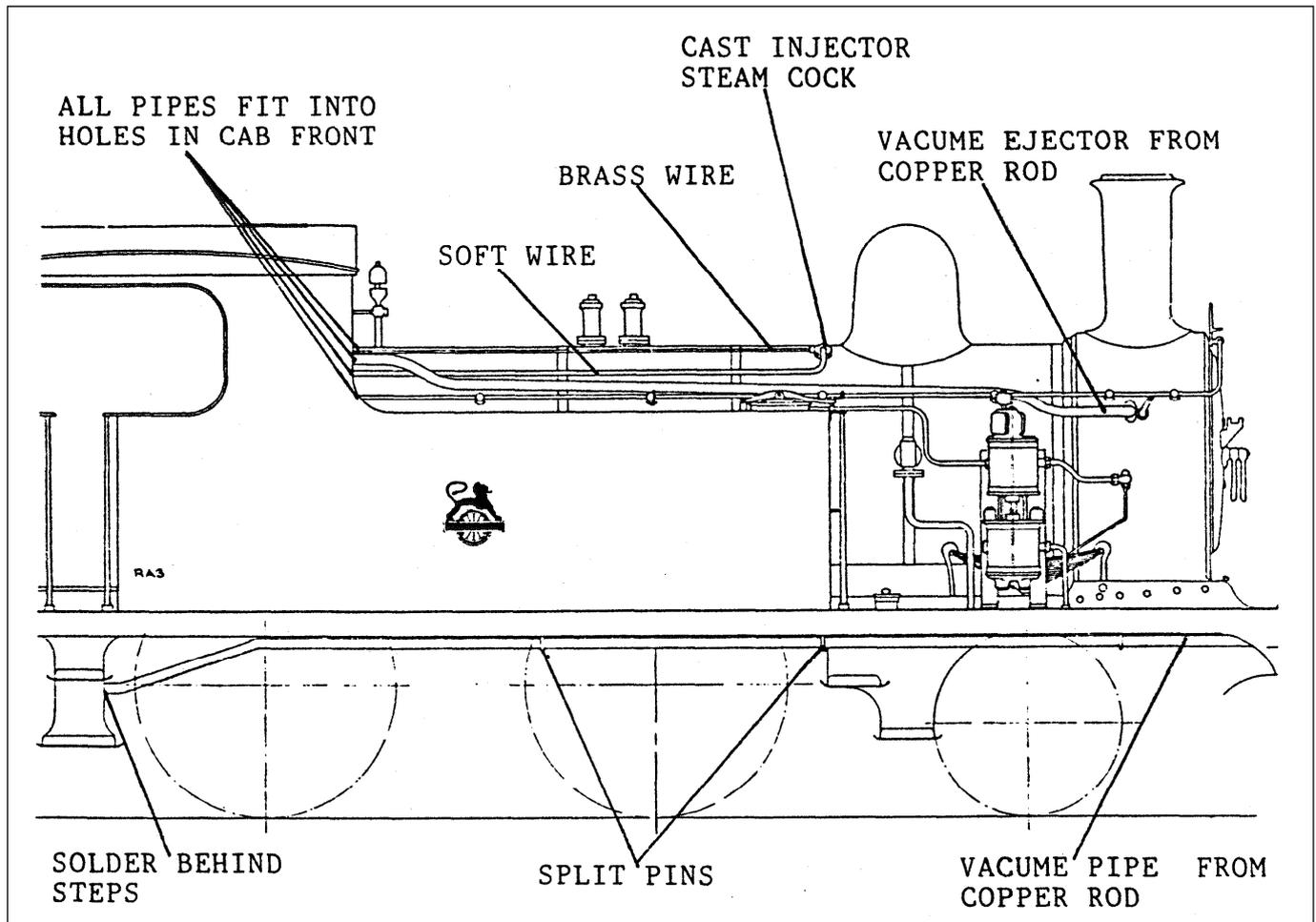
Fit westinghouse pump casting. Drill out holes for pipework. Fit bottom drain pipe. Then fit casting to bracket. Fit the two top pipes made from soft wire.
