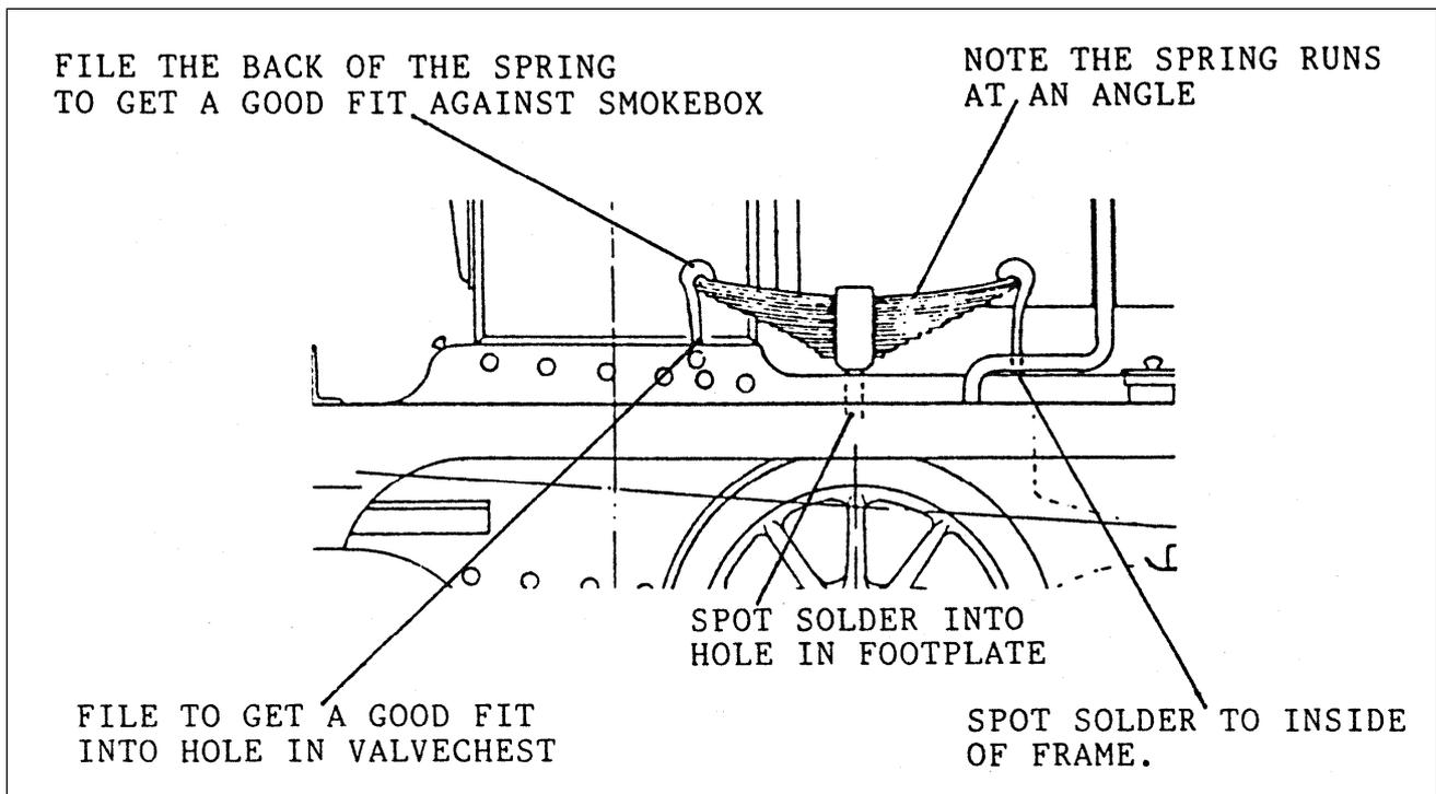
40. WESTINGHOUSE PUMP BRACKET. Fold over top section 180° (to space it from the boiler). Solder it to the footplate and boiler side. See drawings for position.
