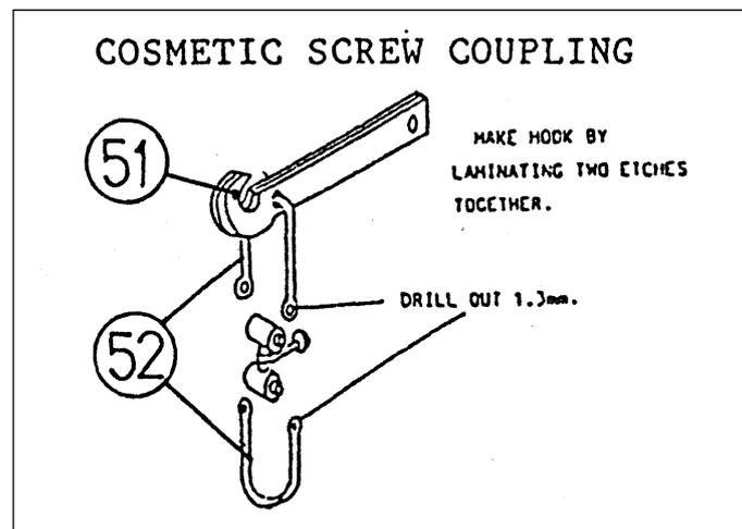
51. COUPLING HOOKS. Laminate two etches together.
