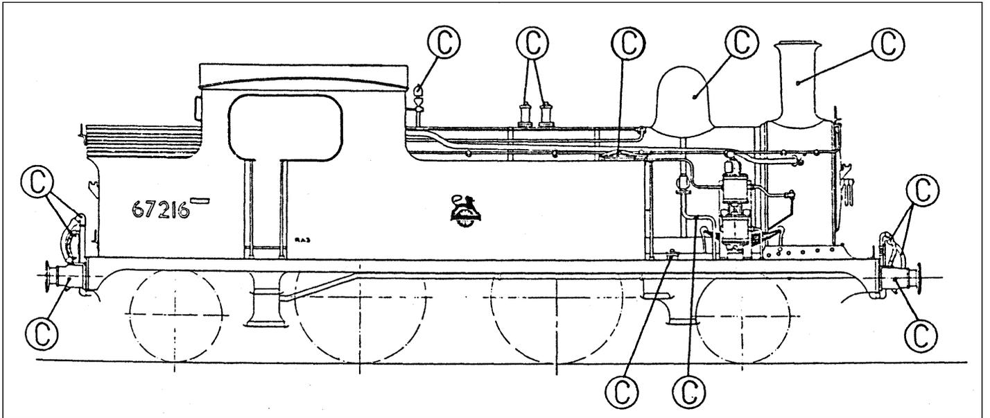
Fit remaining castings with reference to drawing
