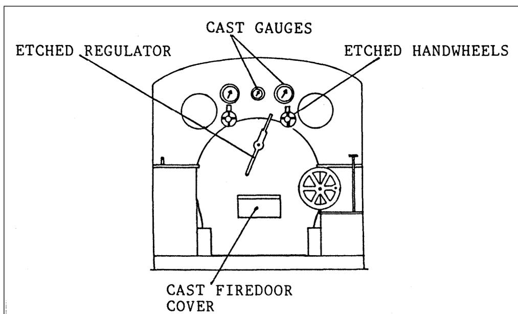
Fit backhead detail and cast gauges to cab front.
