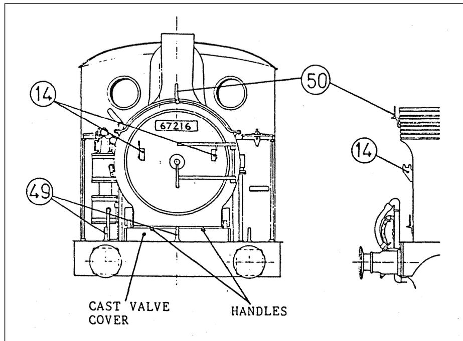
Fit smokebox door casting. Drill out hole in centre and fit door handles. Fit cast valve cover. Drill out holes in casting and fit handles made from track pins.
