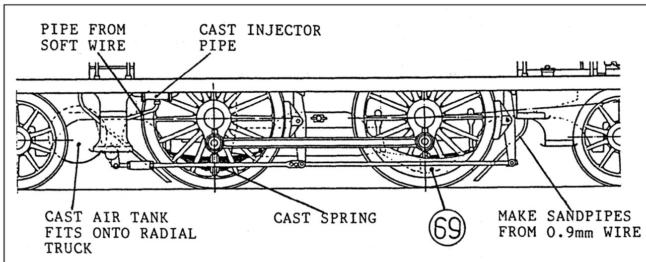
69. WHEEL BALANCE WEIGHTS. Glue to spokes. Now fit remaining castings and detail with reference to the drawings. Note the springs are a standard casting and will need to be chopped a bit to fit to the frames
